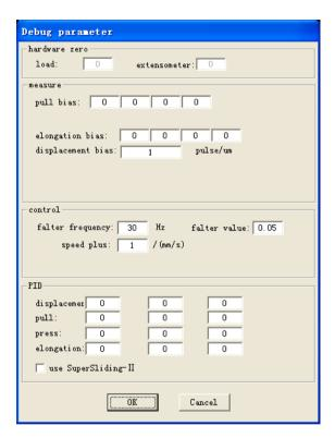
Select the option [Debug parameter] under the [Debug] menu, the diagram of the debug parameter window shows up, the window mostly shows the parameters about hardware zero, measure, control, and PID control, the parameters could also be directly modified here
