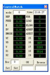
Select the option [Test/Control Watch Window] under the [Tools] menu, the diagram of the Test/Control Watch window shows up. The window displays the sampling about controls of the test, so that faults could be diagnosed if the test has some accidents.
