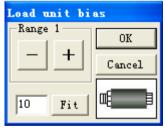
Selects the option "Load bias" in the Menu or press [F8] key to open the tiny adjust the window of the load value, the window shows above;
