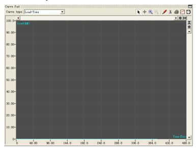
1. **Curve type:** The program would record six different type of curves: Load-Time, Elongation-Time, Load-Elongation, Load-Displacement, Stress-Strain, Load-Strain, these could be switched displaying here;
