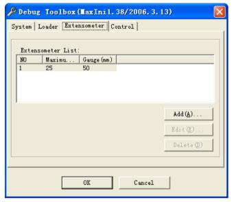
The page is used to add Extensometer.
