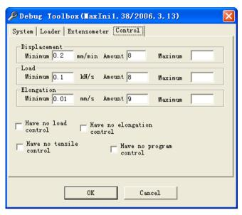
This page is used to customize the control speed of the Displacement, Load, and Elongation. The interface customized shows below:
