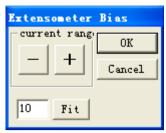
Selects the option "Extensometer bias" in the Menu or press [F9] key to open the tiny adjust the window of the extensometer value, the window shows above;
